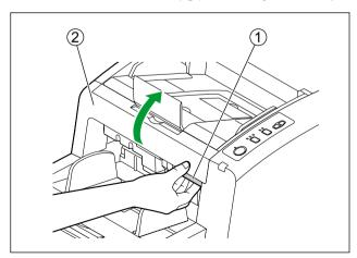
**3.** Move the reference plate lever (R) (1) and the reference plate lever (F) (2).
